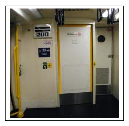
(c) For example, the minimum distance between the centre line of the toilet pan and the far side wall of the toilet module must be at least 1150mm. On an NGR train, this would only leave around 600mm for the
